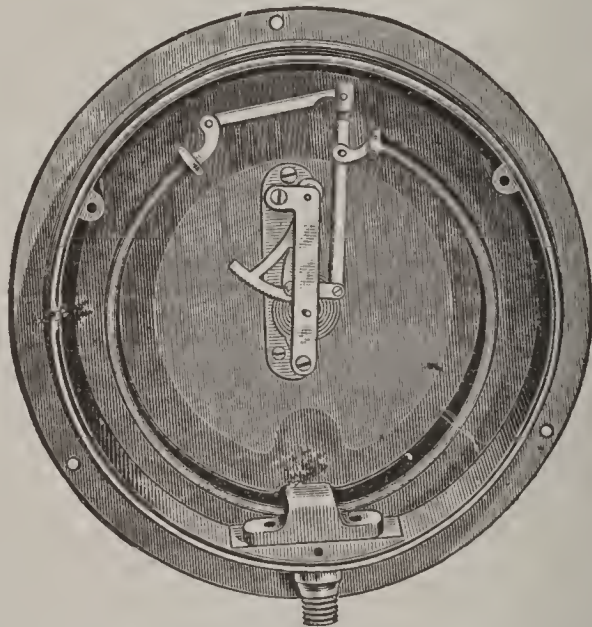
FIG. 75. SECTIONAL VIEW AMERICAN PRESSURE GAUGE.
